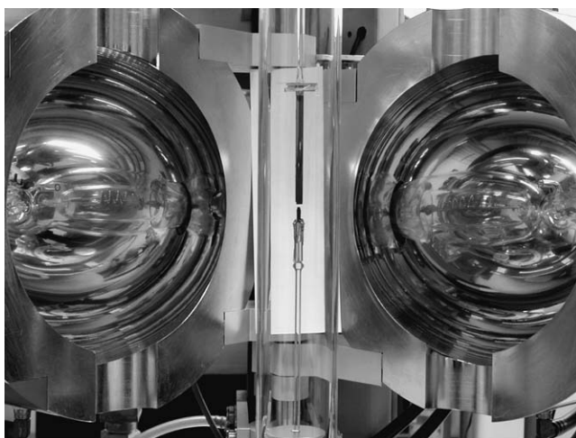
Fig. 5. Photograph of an optically heated floating zone melting furnace with opened elliptical reflectors and loaded with a long and a short polycrystalline sintered rod. The rods are separated from the environment in a gas-tight manner by a quartz glass tube, which acts as sample chamber. The process atmosphere can be chosen by a flow of an appropriate gas through the quartz glass tube. A lamp is located at the outer focus of each of the elliptical reflectors. During operation, the reflectors are closed, i.e. they surround the quartz glass tube completely. Thereby, the radiation from the lamps is concentrated on the inner focus, where the ends of the rods are located. By using a sufficiently high lamp power, the material located in the inner focus can be melted as shown in Fig. 6.
