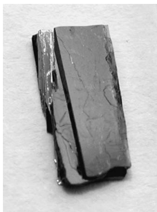
Fig. 7. Photograph of a Sr 2 RuO 4 single crystal obtained by crushing the as-grown sample. The approximate size of this crystal is 2 \times 1 \times 0.2 \text{ mm}^3 .
