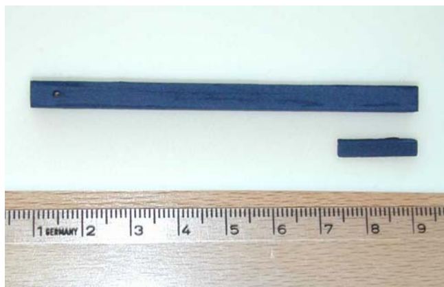
Fig. 18. Photograph of two sintered polycrystalline rods. The length of the long rod is 8 cm.
